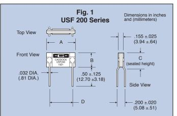
**USF 200 Series Circuit Board Connection Note:** The Type USF 200 Series Resistor must have the two "bonded" resistors in the package connected in parallel on the circuit board as shown. This parallel connection of the two resistors achieves the specified resistance with the specified performance.
