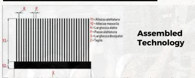
The assembled dissipators are formed by mechanically assembling individual wings, giving them both high dimensional flexibility and the same mechanical characteristics as extruded dissipators. However, by focusing on the section of a single wing, the number of wings and their arrangement can be adjusted to make them ideal for high-power systems with forced convection.
