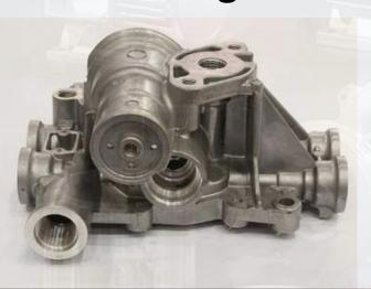
At MG Italia, we utilize CAD systems to guarantee precise flow analysis during casting, ensuring top-notch quality. Our laboratory is equipped with the capability to completely automate the milling process, tailored to meet the specific requirements of each customer.
