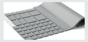
Nolato's own manufactured range of Thermal materials, available with low MOQ's and from stock. Sheet sizes start at 0.3mm thick and standard overall size is 200mm x 200mm. Larger sheets available on request.
