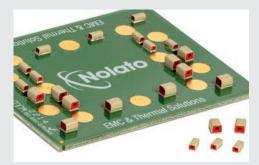
Excellent mechanical properties, large conformable contact area vs metal spring. Full, strong chemical bondage between gasket and metal. No Scratching of PCB. SMT
