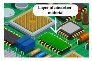
With their high magnetic absorption losses ( $\mu$ ") and magnetic field storage capacity ( $\mu$ '), these plates reduce the noise caused by the radiating component.
