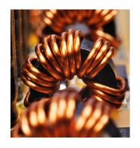
Sintering NANOMAG-MnZn enables to realise magnetic components used in inductors, transformers and converters.
