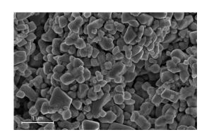
NANOMAG-MnZn is a Manganese-Zinc (Mn,Zn)Fe<sub>2</sub>O<sub>4</sub> ferrite powder.
