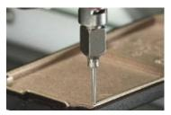
Dispensed gasket, precisely applied by a dispensing nozzle under CNC control to enable continuous application of intricate, small cross section gaskets.
